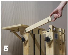
Secure the laterals, with the Velcro facing inwards and the open slot to slip onto the screw and wingnut of the back.
