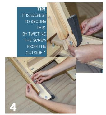
Position the table by removing the provided screw and wingnut, selecting the desired setting and securing the screw and wingnut.\*
